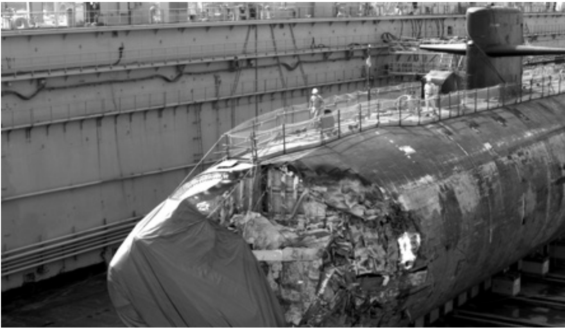
Since submarines “see” by sonar, their bows (where the sonar is located) are made of plastic. Plastic does not respond well to sudden impact, as evidenced by this photo of the USS San Francisco, which hit an uncharted underwater mountain in 2005 while travelling at full speed.
